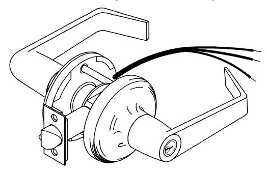
TERMINATE THE WIRES FROM LOCK TO THE ELECTRIC POWER TRANSFER DEVICE USING 22 AWG WIRE. USE PROPER CRIMP SPLICES OR WIRE NUTS FOR TERMINATING CONNECTIONS.
