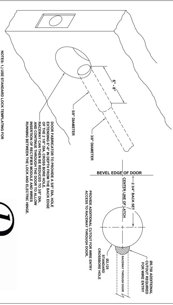
DOOR PREPARATION. PROVIDE ADDITIONAL PREPAS SHOWN FOR ELECTRIC LOCK MODIFICATIONS
