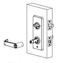
11:Slide inside lever onto spindle and lock it into place, tighten two mounting screws being careful not to over tighten. Check to see if rotation is smooth and if function is correct.
