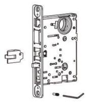
2. Pull latch bolt out of lock
