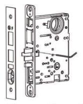
1. Remove special screw with provided allen wrench
