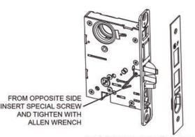
Reinstall the special screw and tighten securely with the provided allen wrench.
