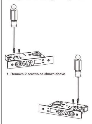
Turn lock over to opposite side and reinstall screws as shown above.
