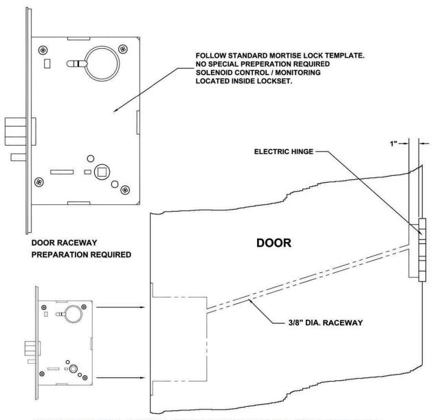
DOOR FABRICATOR TO PROVIDE A 3/8" DIAMETER (MINIMUM) RACEWAY THROUGH DOOR TO ALLOW THE INSERTION OF ELECTRICAL WIRES RUNNING BETWEEN THE LOCK MORTISE AND THE ELECTRIC HINGE.
