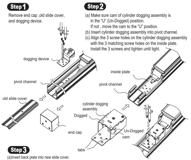
(b)Install cylinder collar onto the mortise cylinder and insert into new slide cover and back plate. Then, thread cylinder retaining ring onto cylinder until finger tight.
